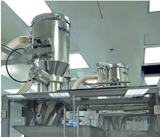
Loading a tablet packaging machine.
