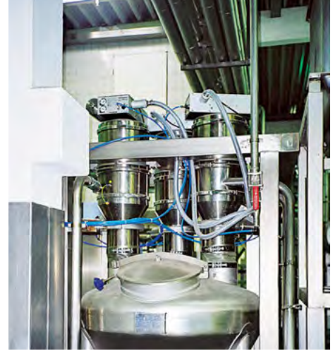
Conveying of cake/bread mixtures in the food industry.
