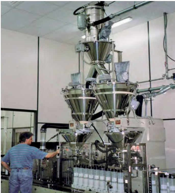
Loading a toner filling system.
