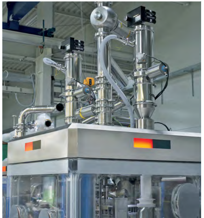
PPC with a WIP function on a table press.
