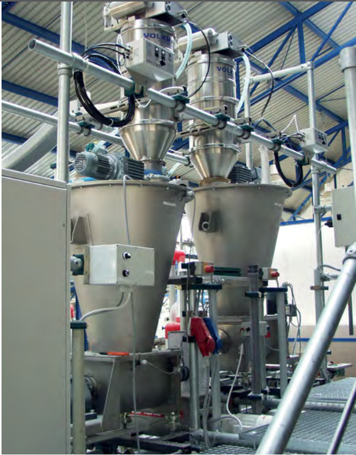
Two vacuum conveyors for loading loss-in-weight feeders.
